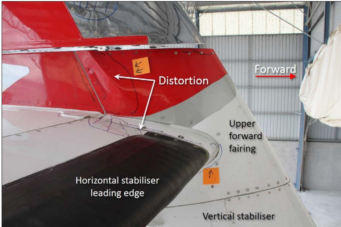
Figure 6: Distortion in the upper forward fairing right side horizontal stabiliser leading edge prior to removal of any fairings or access panels.
