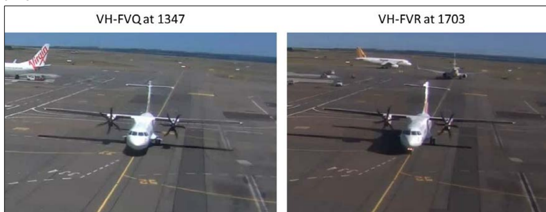
Figure 5: Images from Sydney Airport CCTV footage showing the deformation to the horizontal stabiliser of VH-FVR (right) as compared to an undamaged ATR 72, VH-FVQ (left).
