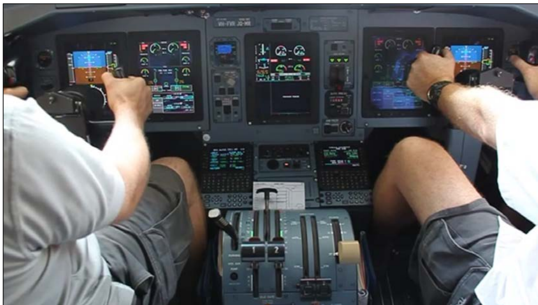
Figure 47: Still image from video of on-ground pitch disconnect testing carried out on VH-FVR following the occurrence. The right control column was held fully forward while the left control was pulled back. The image is just before the pitch uncoupling mechanism activated. Note the difference between the left and right control column positions. The left control column is about halfway through its full travel, while the right control column is at the forward limit.
