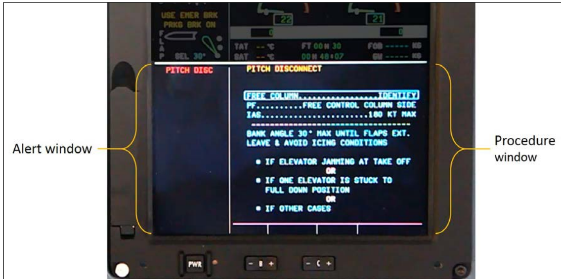
Figure 24: The bottom half of the engine and warning display is dedicated to the flight warning system. The alert window, on the left, lists all of the active alerts. The procedure window on the right automatically presents any procedures associated with the active alert. The pitch disconnect warning is provided as an example.
