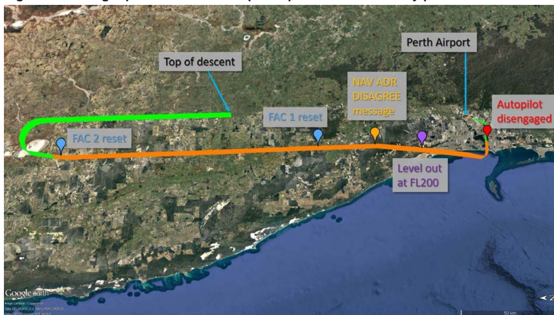
Figure 3: The flight path from take-off up to top of descent with key points identified
