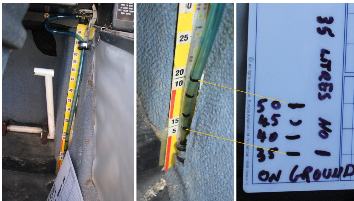
Figure A3: Fuel quantity scale located behind the fuel sight gauge. Four black marks correspond with the Pilot Check Card marks and figures that were developed following pilot B's fuel calibration.
