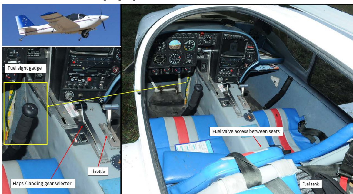
Figure 1: VH-BWI and cabin interior showing component locations. Note the instrument panel and fuel sight gauge orientation toward the left pilot. Refer to Appendix A for further detail on the fuel sight gauge.
