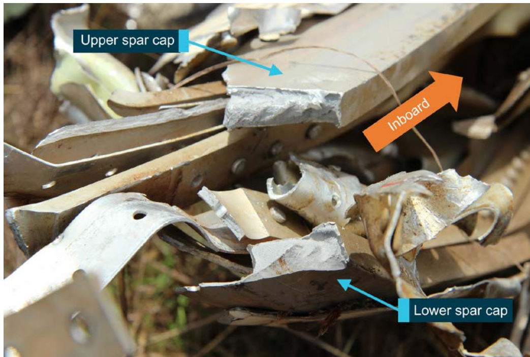
Figure 8: Fractured main spar caps from the right wing
