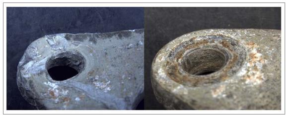
Left: bolt-hole for the missing fastener. Right: bolt-hole for a removed fastener. Source:  $\ensuremath{\mathsf{ATSB}}$
