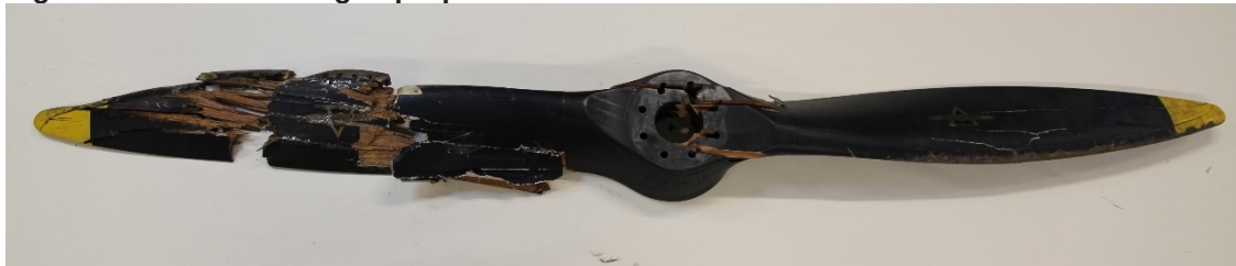
Figure 5: VH-UZB damaged propeller
