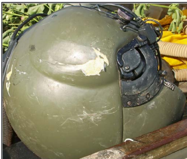
Figure 3: Damage to the left side of the pilot's flight helmet
