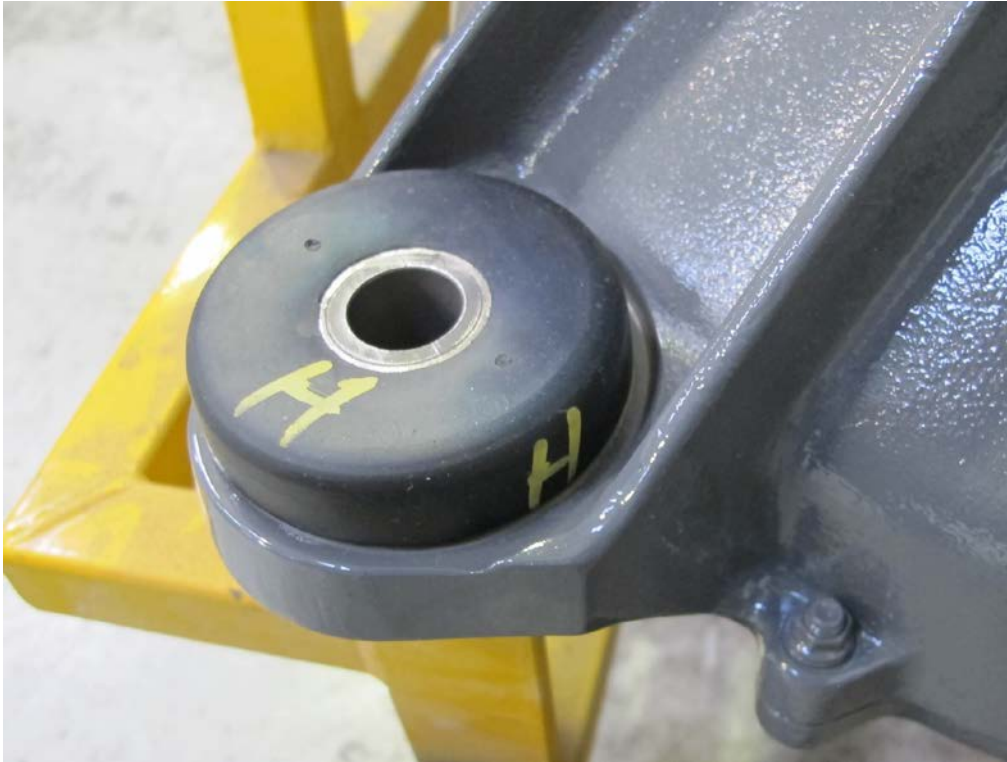
Figure 2: A653-2 gearbox mount installed
