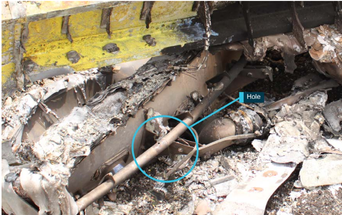
Figure 10: Gate box wreckage showing hole in gate box torque tube where bolt was missing
