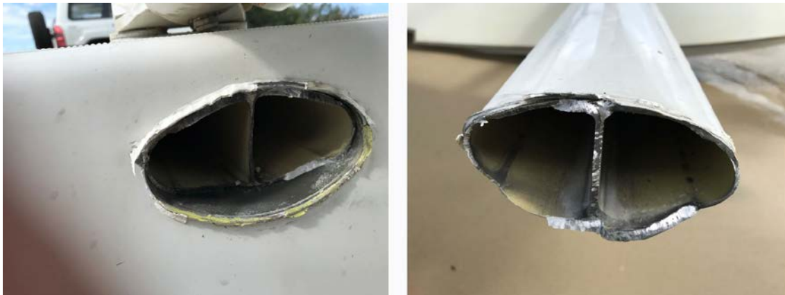
Figure 3: Front spreader bar fatigue failure located within the float
