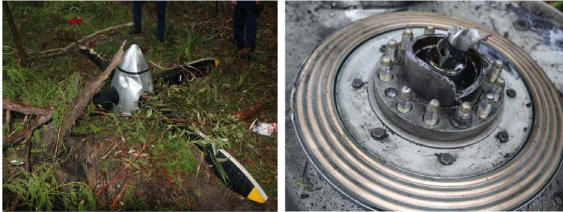
Figure 2: The separated propeller from VH-NRX
