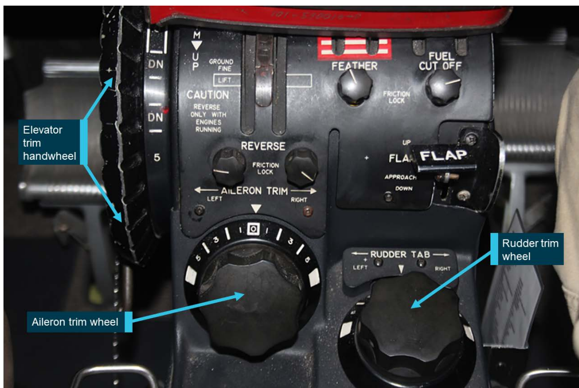
Figure 4: Position of the elevator trim wheel, aileron trim wheel and rudder trim wheel on the centre pedestal of a B200 aircraft
