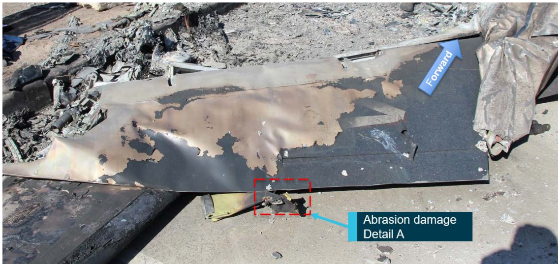
Figure 32: Rudder and rudder trim showing abrasion damage
