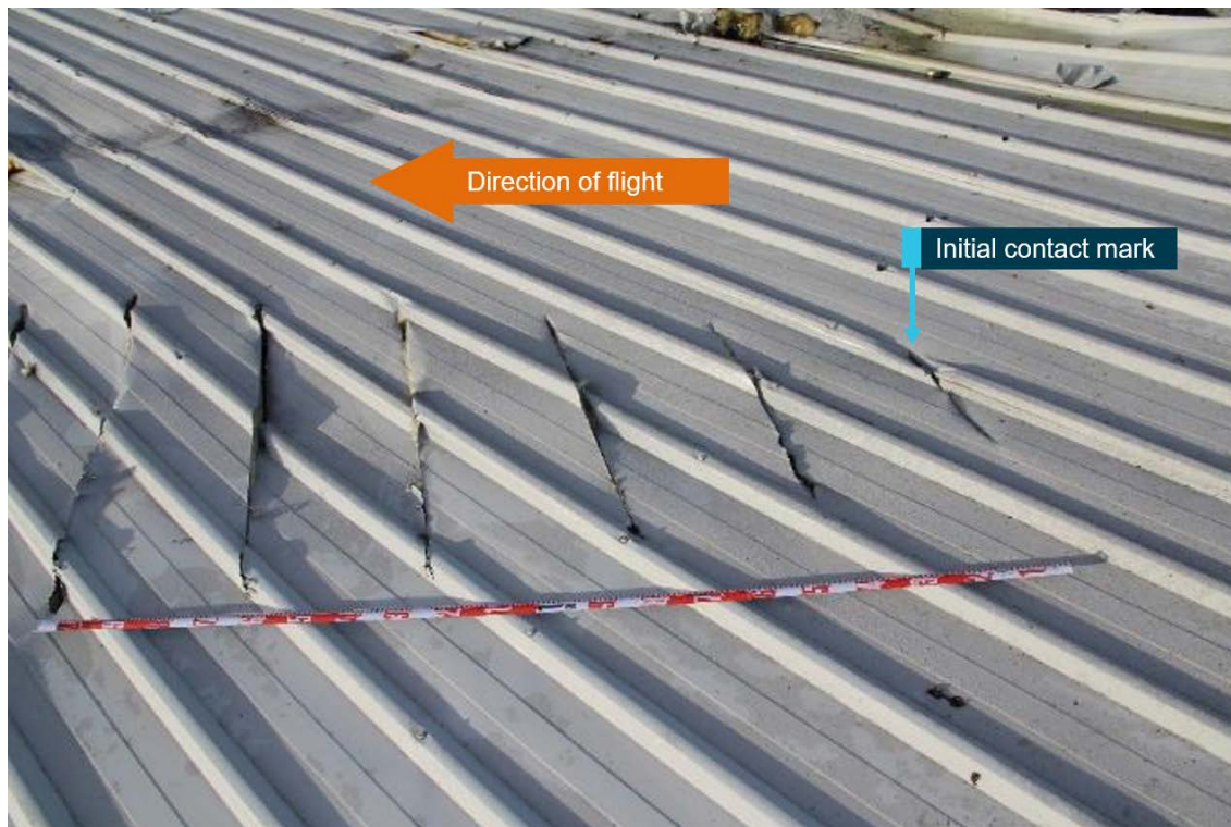
Figure 27: Left propeller slash marks in roofing material with tape measure showing distance between cuts
