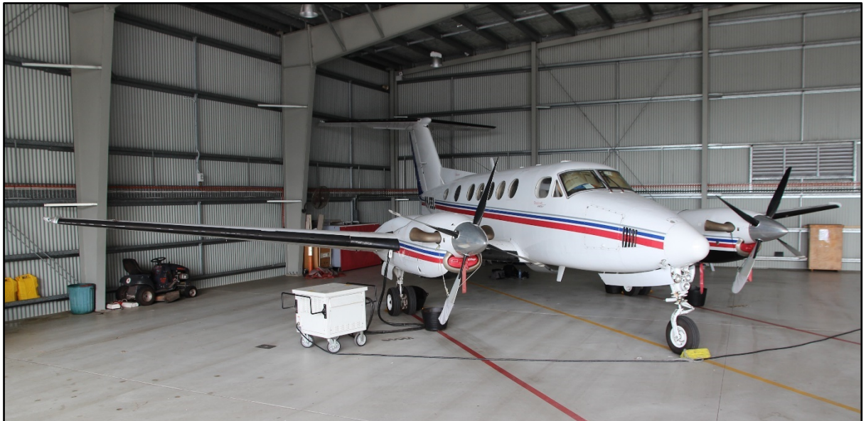
Figure 40: Image of exemplar aircraft taken at an angle of 30° showing the increase in engine cowl fuselage and vertical tail surface that would be exposed to the relative airflow with a sideslip of 30°
