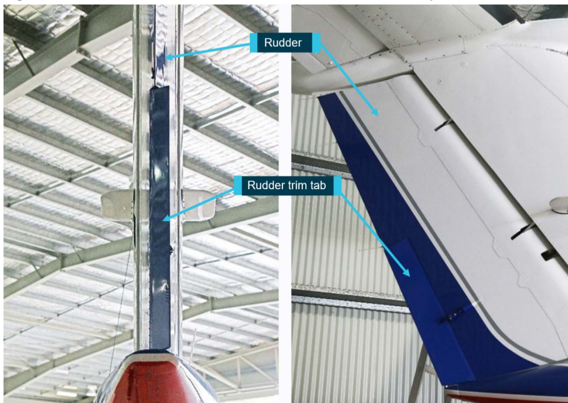
Figure 42: B200 rudder with rudder trim tab set to the full nose-left position
