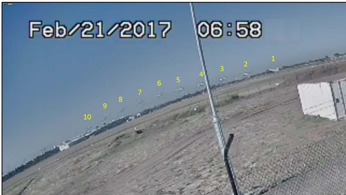
Figure 23: Time-lapse CCTV image of the ZCR's flight path, with images taken every second
