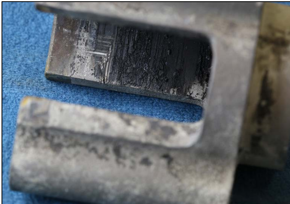
Figure 53: Abrasion damage to the housing attributed to sliding contact from the right cable
