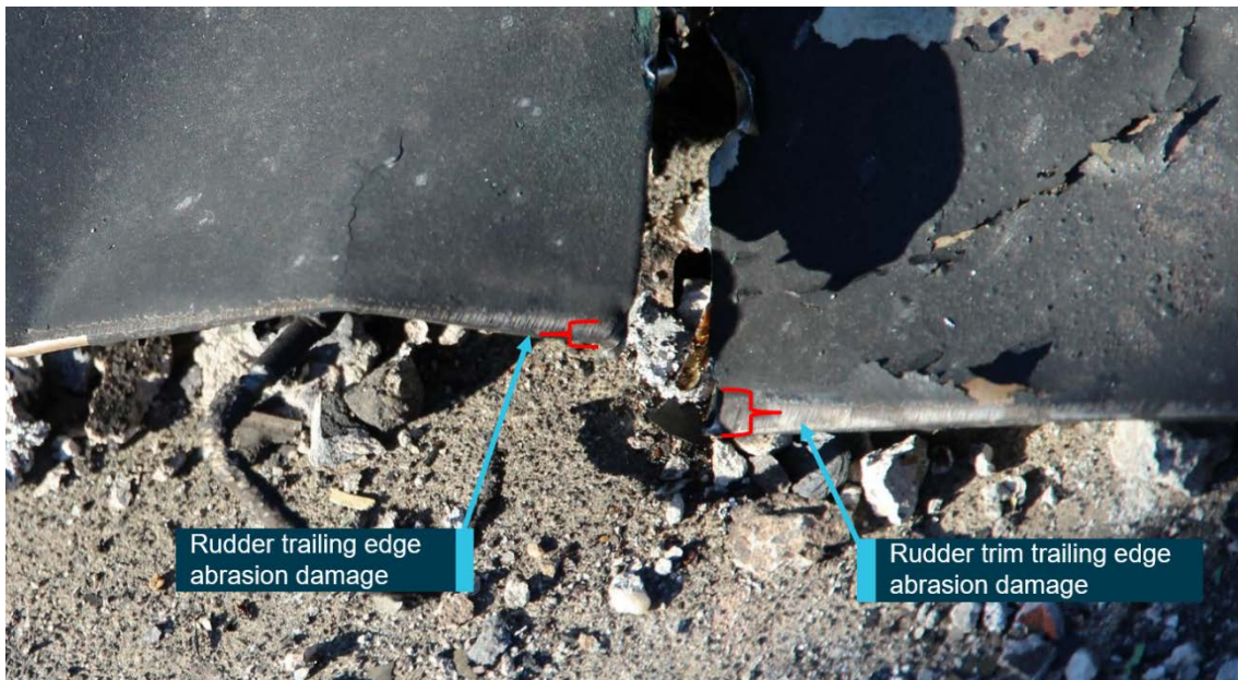
Figure 33: Detail A. Close-up of abrasion damage to rudder and upper surface of rudder trim trailing edge
