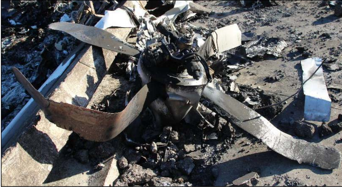
Figure 36: Left propeller viewed from the rear, showing blade-tip fractures, blade gouges and blade bending
