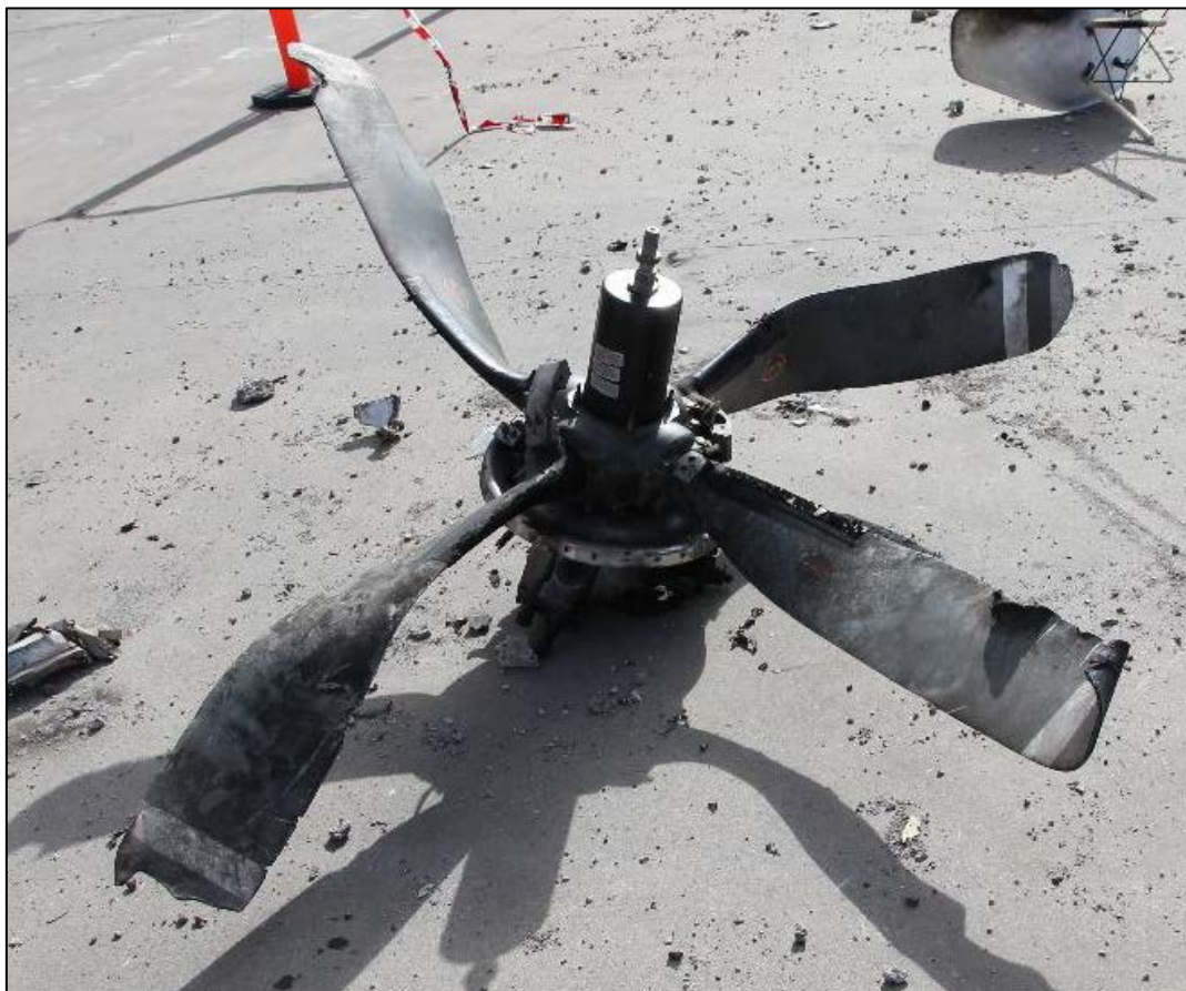
Figure 38: Front view of the right propeller showing bending, chordwise twisting, and leading edge gouging of the propeller blades
