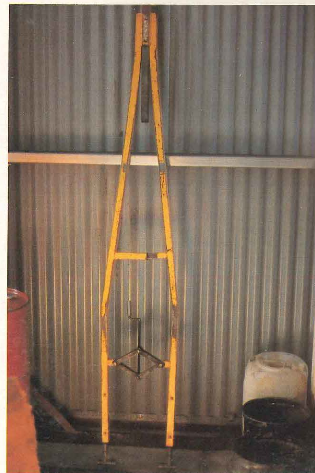
Rigid towbar used for power towing during maintenance operations.
