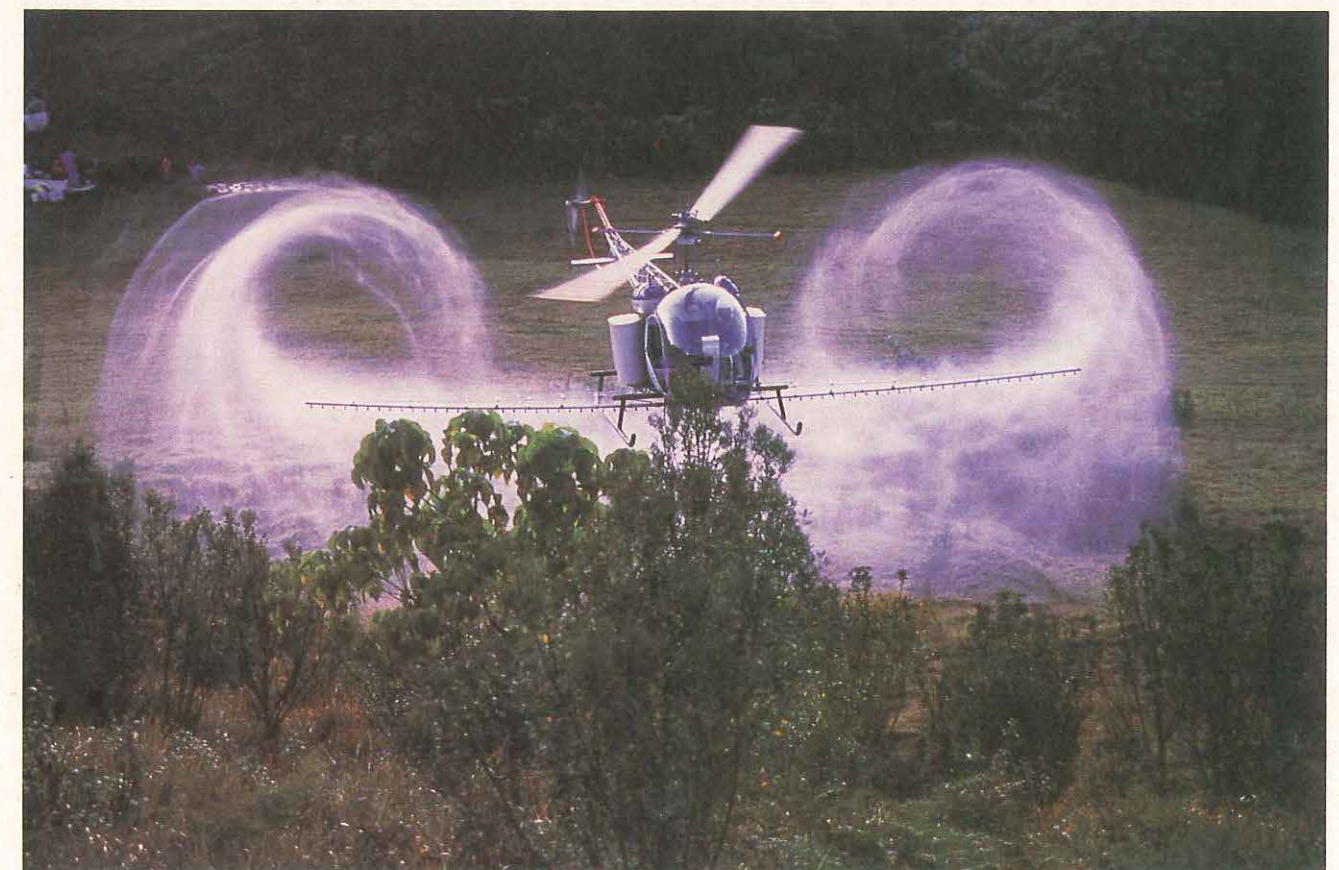
Main rotor vortex from a Bell 47G engaged in agricultural spraying
