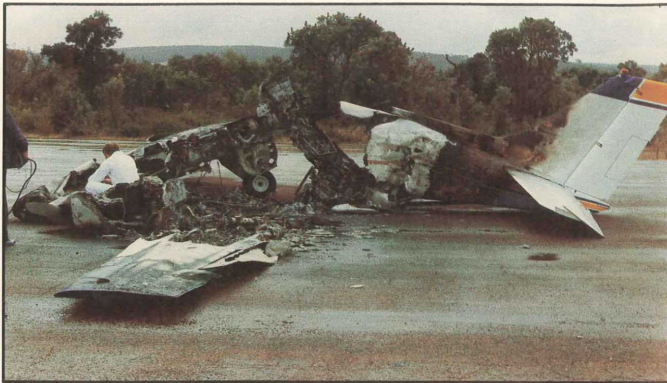
This light twin was destroyed by fire after the extinguisher was found to be unserviceable.
