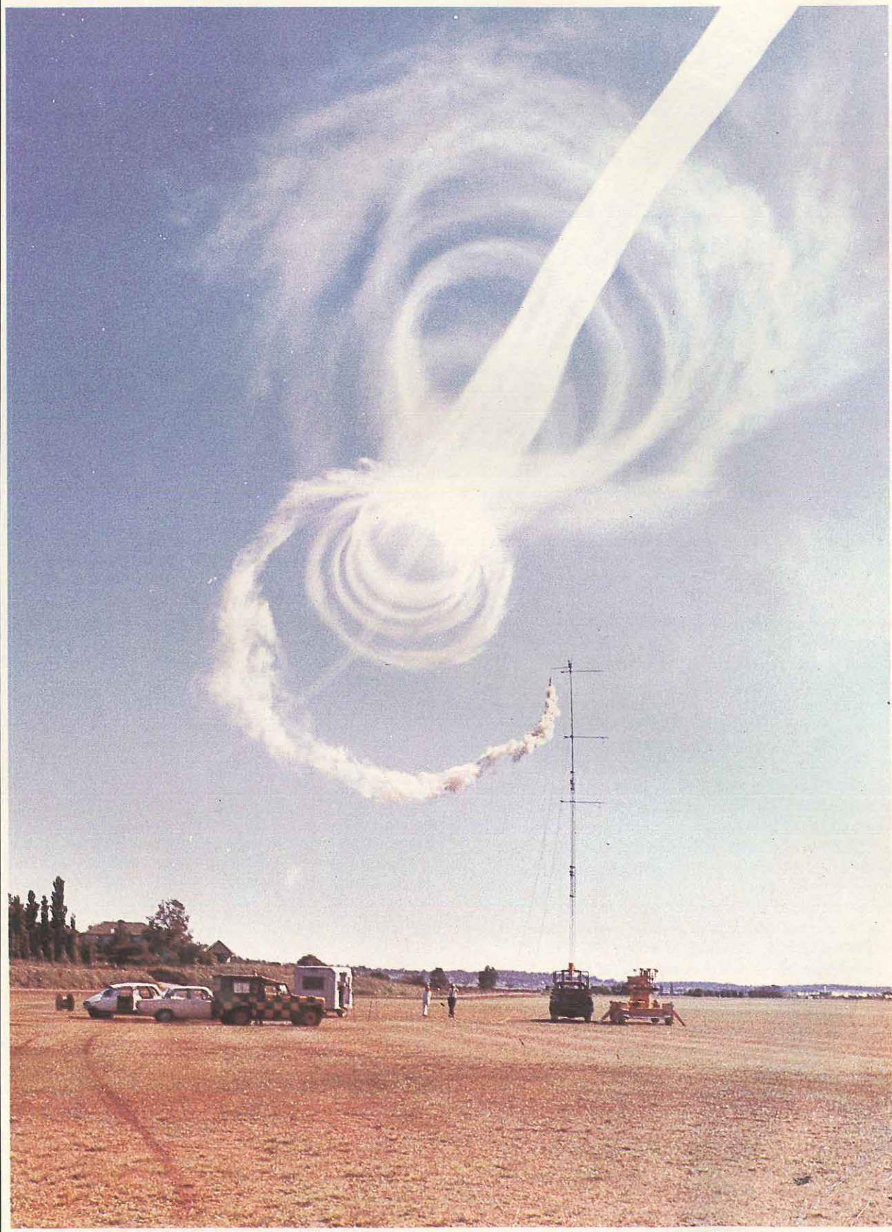
A Lockheed Hercules flew through smoke from a smoke generator fixed to a mast to produce this visible wingtip vortex. The intensity of the vortex is obvious.
