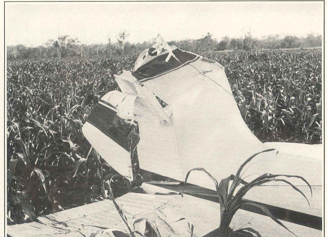
Tail section of the aircraft. Note the primary and secondary failures of the fin. Horizontal stabiliser and elevator damage was caused by ground impact.
