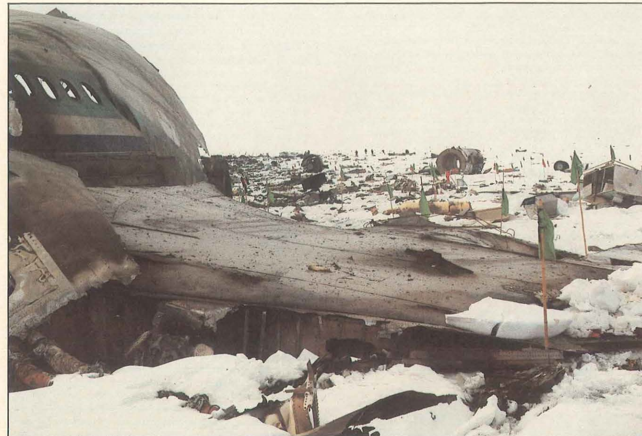
Wreckage of Flight 901 was scattered over a wide range of the ice and snow-covered slopes on the northern side of Ross Island after ground impact. All 20 crew members and 237 passengers on board were killed in the accident.
