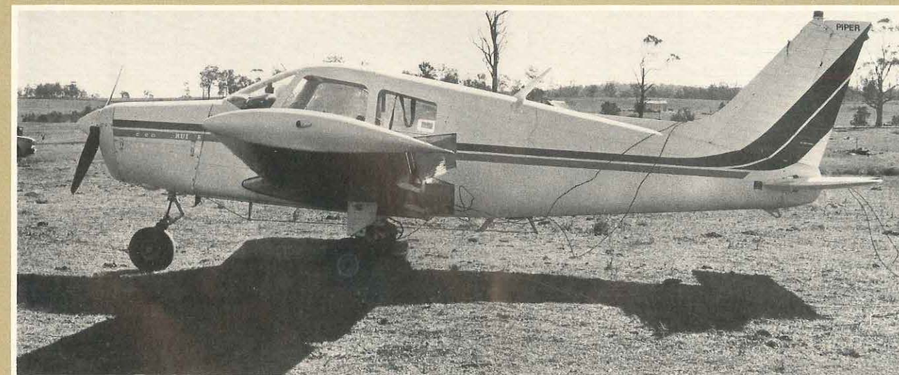
The aircraft as it came to rest. Broken power lines are shown wrapped around the left undercarriage, rear fuselage and right stabilator.
