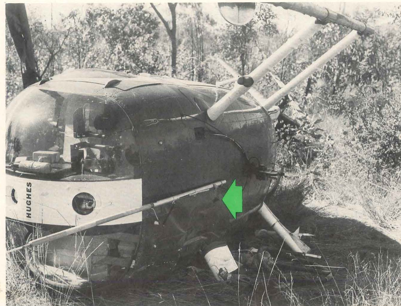
Underside of the wreckage showing the location of the lower vent fairing
