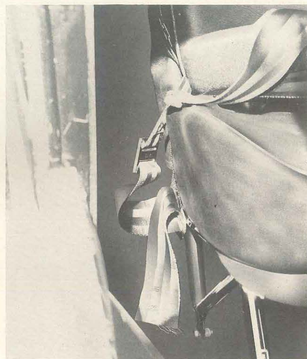
The photograph above shows the harness as found on a Bellanca. Note the limited accessibility, and the fact that this is on the more accessible side, adjacent to the large entry door. The free end of the strap should be passed back through the adjuster, which is too far up from the end fitting.
