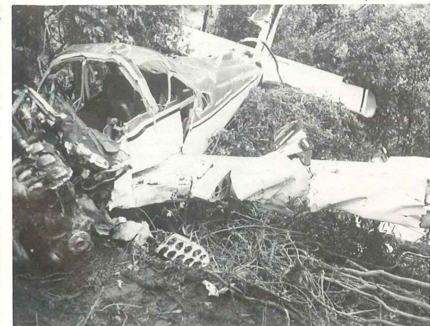
The wrecked aircraft lying on the hillside in dense undergrowth. Impact damage to the cabin area was less severe than the picture indicates as it was necessary to cut into the wreckage to extricate the occupants.
