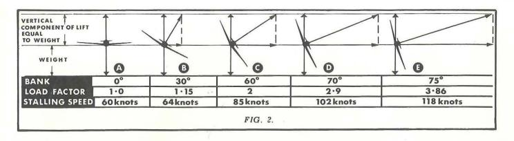
the wings be increased to maintain height. The resulting increase in dynamic load will therefore cause an increase in stalling speed. Thus one of the essential facts of flight that should always be to the fore in the speed increases in a turn.
