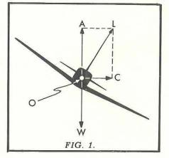
of course vertical in straight and level flight, but now is inclined to the vertical at the angle of bank. The vertical component OA of OL, balances the weight of the aeroplane, while the horizontal component OC of OL provides the necessary centripetal force.
