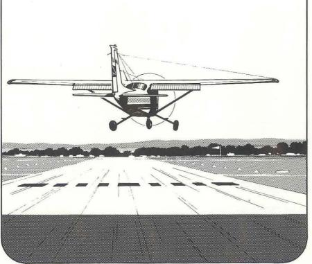
maintain rudder effectiveness. Then, when the aircraft is tracking straight down the runway, the upwind wing is centre line of the aircraft. But on lowered smoothly to prevent further drift and the hold-off continued until the upwind wheel touches the ground. After touchdown, the aircraft is kept straight by using a combination of rudder and upwind aileron.
