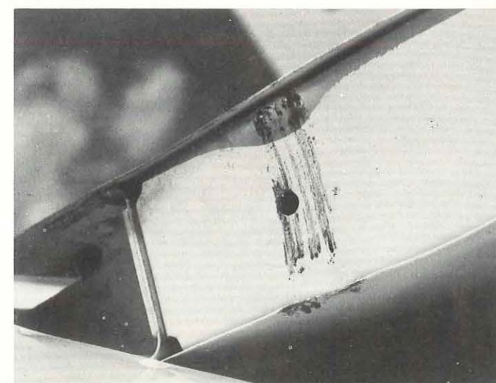
Close-up of outboard edge of starboard tailplane showing score marks made by cinder jammed between tailplane and elevator horn. The buckled lower skin of the tailplane was partially straightened by an engineer before the photograph was taken.
