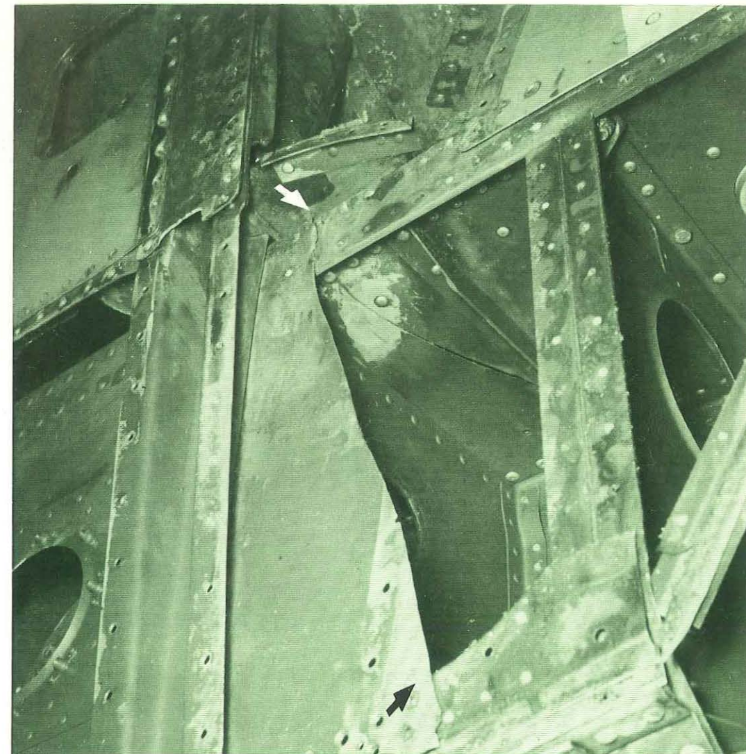
Figure 1: View from underside of wing looking forward, showing cracked main spar web and failed lower spar cap. The rear section of the lower nacelle structure and most of the wing skin has been removed. Note also the fracture in the wing skin panel which had been hidden by the nacelle fairing.
