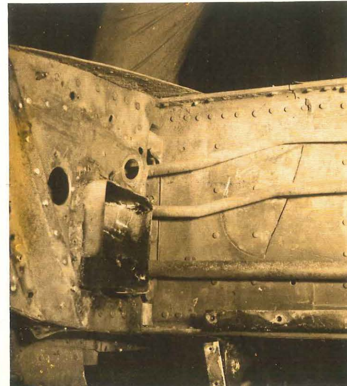
Figure 2 — Left: Another view from underside of wing showing fractured wing skin panel. Note scorching and charring of skin in vicinity of spar cap failure at top of picture. The engine support beam had been removed before this picture was taken.
