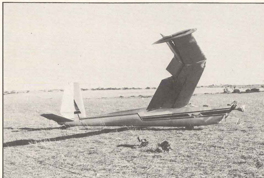
Bottom: The distortion of the nose section as seen in this picture indicates the attitude of the Blanik at impact.
