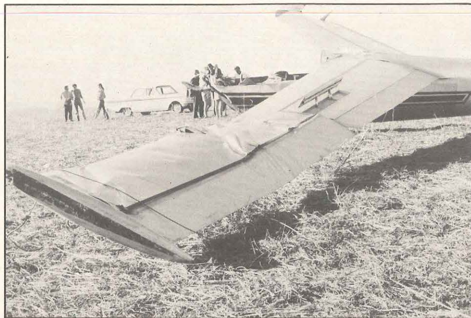
Top: The main impact was also taken on the glider's port wing. This close-up shows the severe distortion and wrinkling of the wing structure.
