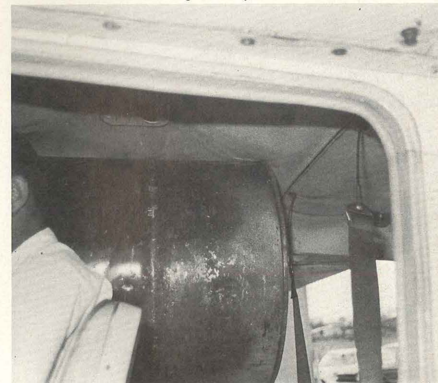
Below: With the aircraft loaded in this manner, it was not possible to secure the drums to the cargo tie-down points.
