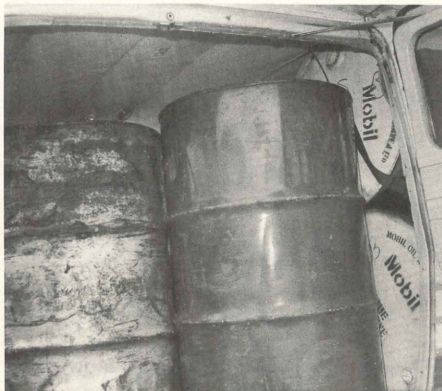
Reconstruction of aircraft loading at time of accident. Above: View taken through main door of aircraft showing relative position of drums. The fifth drum is on its side in the rear of the cabin just out of the picture to the left.
