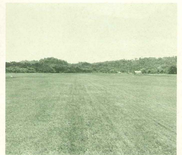
View taken from centre of Aitape airstrip looking north towards upwind end. After commencing to go around, the pilot apparently realised he would be unable to out-climb the hills in the background. The river in which the aircraft crashed is amongst the trees on the left of the picture.
