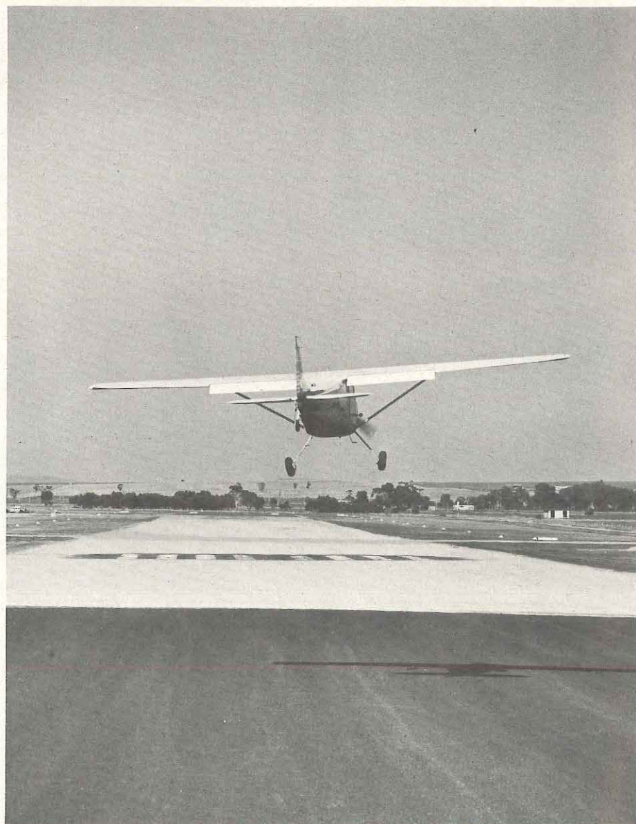
The "crabbed" approach, with the aircraft headed slightly into wind so that its approach path is aligned with the runway.
