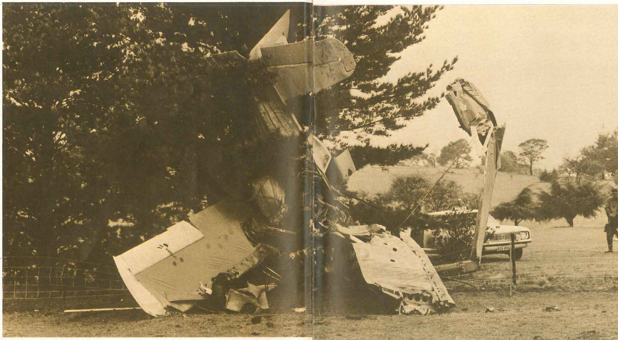
Wreckage of the Grumman Agcat as it came to rest on the golf course boundary after diving into the ground out of control.
