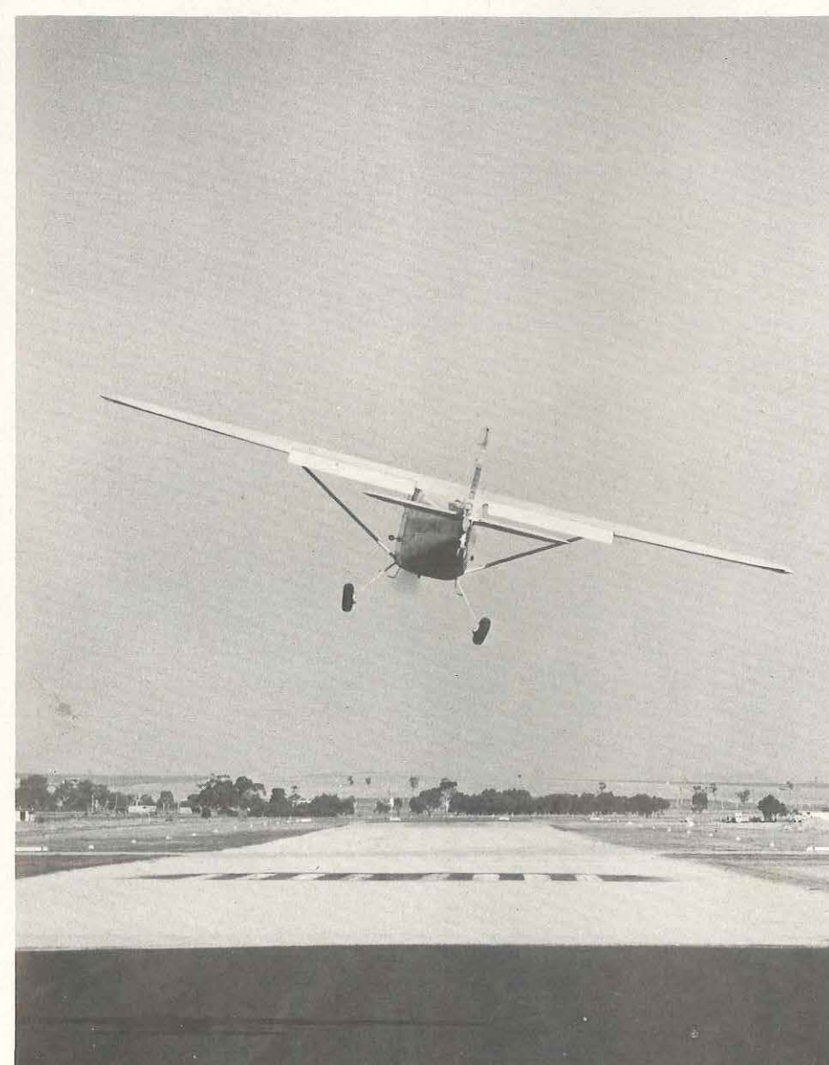
The side-slipping approach. In this case, the effect of the side slip counteracts the drift produced by the crosswind.
