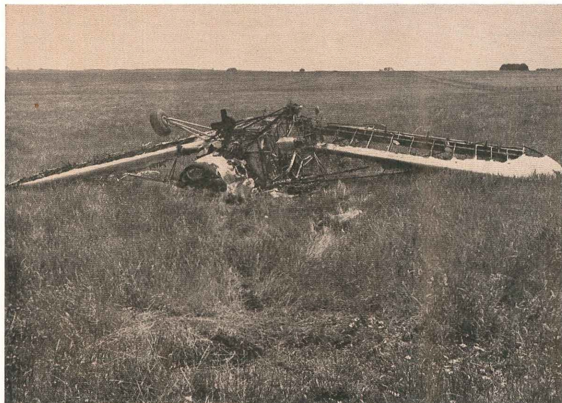
Above: The burnt-out wreckage, looking in the direction of flight. The landing strip can be seen on the rising ground directly behind the aircraft. The point of initial impact is in the foreground, indicated by the circle of grass cut by the propeller.
