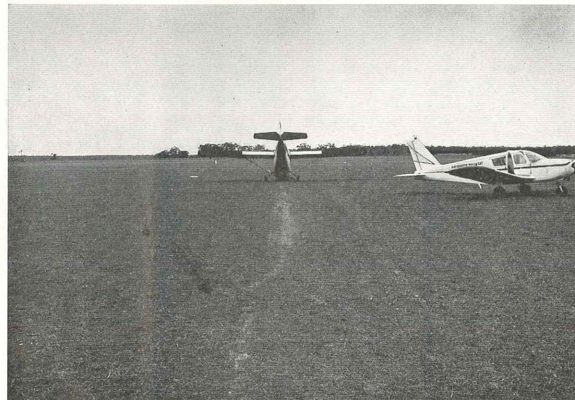
Below: The damaged aircraft, as it came to rest on the strip looking in the landing direction. Ground marks left by the underside of the engine cowl as the aircraft slid to a halt, can be seen in the foreground.
