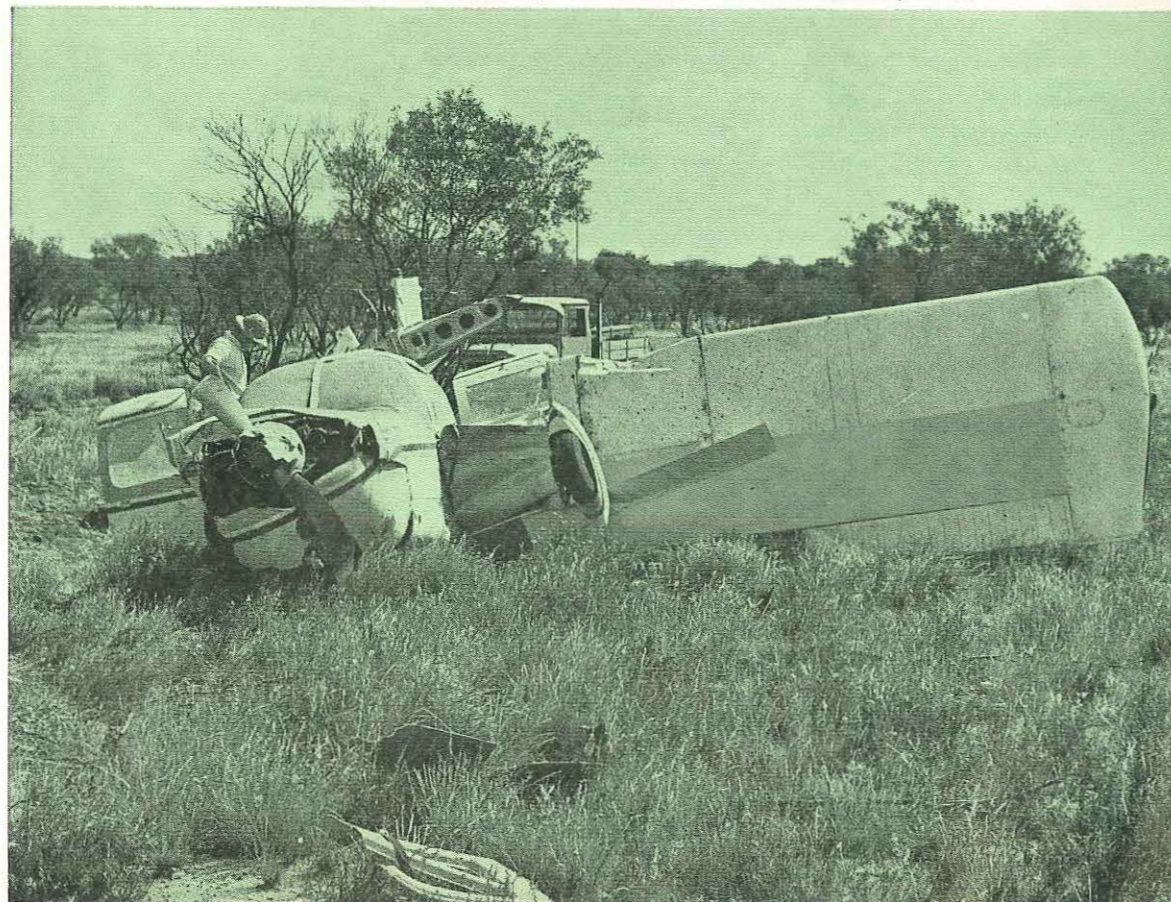
The aircraft as it came to rest alongside the Hermannsburg-Alice Springs road. Although both wings were torn bodily from the fuselage the cabin area remained relatively intact.
