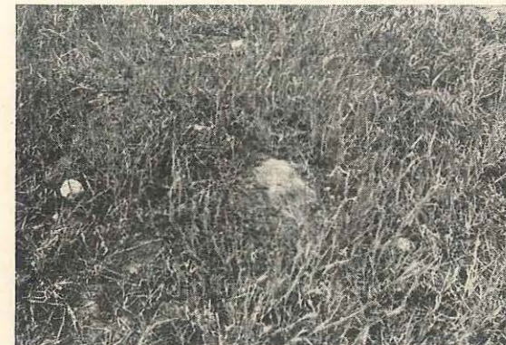
Long grass in the paddock from which the aircraft was operating almost obscures the rock struck by the nose wheel.
