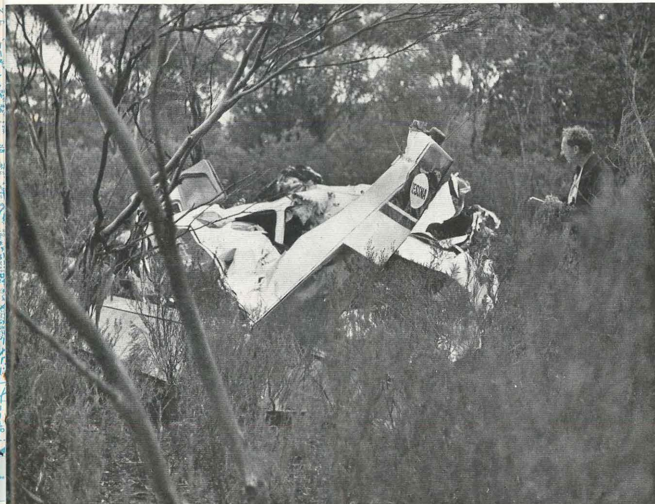
The wreckage as it was found. The lack of damage to the surrounding undergrowth clearly indicates that the aircraft struck the ground in a near-vertical descent.
