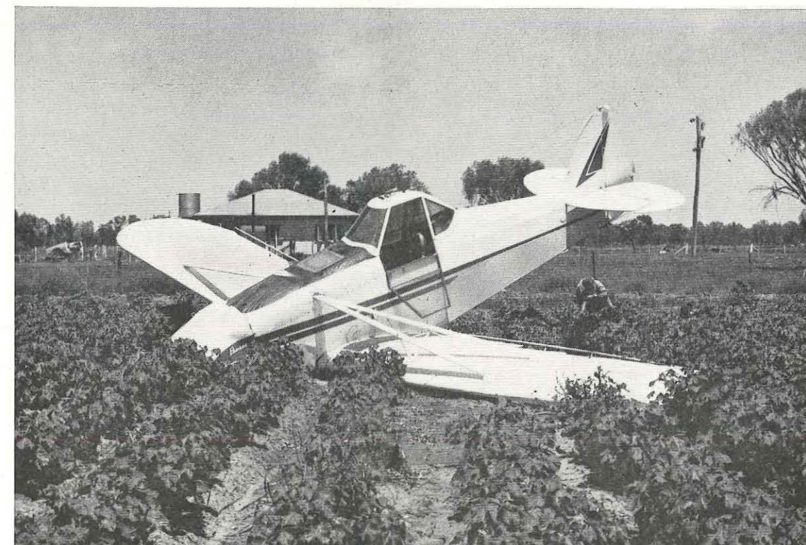
The privately-owned Pawnee as it came to rest after flying into the second power line. Portion of the line can be seen in the background.
