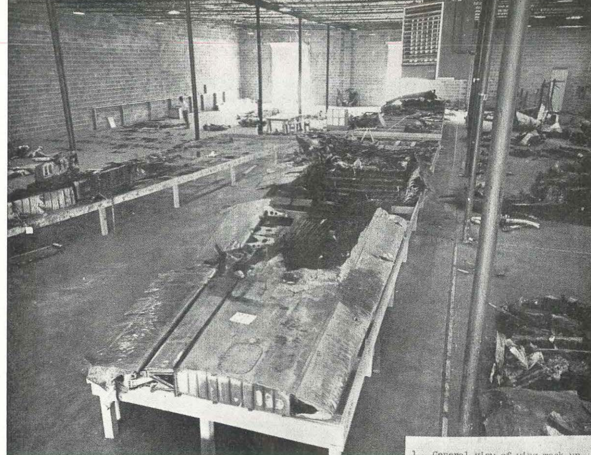
The wreckage of the Electra's wing being "reconstructed" during the investigation.
