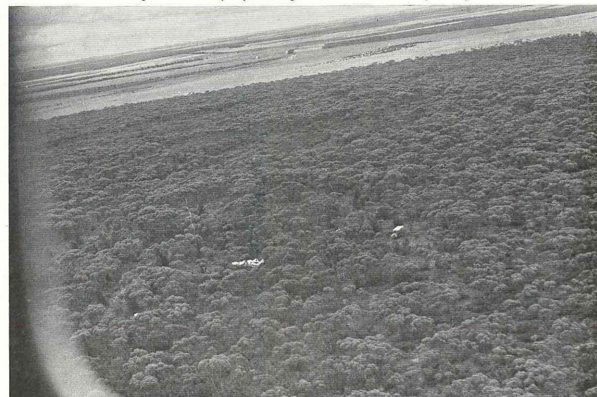
Aerial view of accident site looking back in direction from which aircraft had come. Note the complete absence of any wreckage trail in the surrounding undergrowth.
