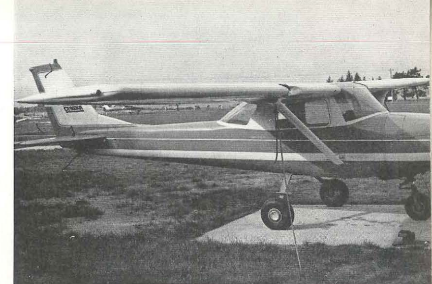
Above: The Cessna 150 after it had returned to the aerodrome. Note the hole in the leading edge of the starboard wing.
