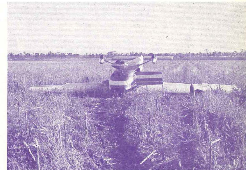
The ridge of earth which forced the nose wheel off-centre. The path of the deflected nose wheel through the soft soil is clearly evident.
