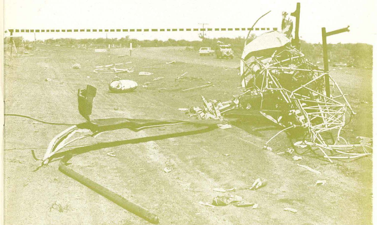
General view of the wreckage with the position of the stay wire indicated by the heavy dotted line. The damaged anchor point shown on the opposite page can be seen at the extreme left. The picture was taken looking back in the direction of the helicopter's approach.
