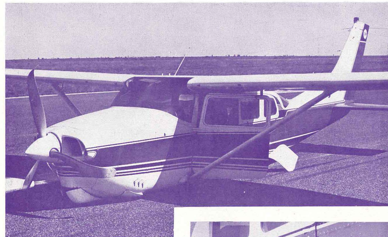
These pictures show clearly that the undercarriage extension cycle had begun before the aircraft landed. The nose wheel doors are half open and the port main undercarriage door is fully open. Insufficient fluid in the hydraulic system prevented completion of the cycle.
