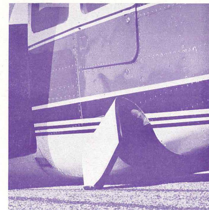
These pictures show clearly that the undercarriage extension cycle had begun before the aircraft landed. The nose wheel doors are half open and the port main undercarriage door is fully open. Insufficient fluid in the hydraulic system prevented completion of the cycle.
