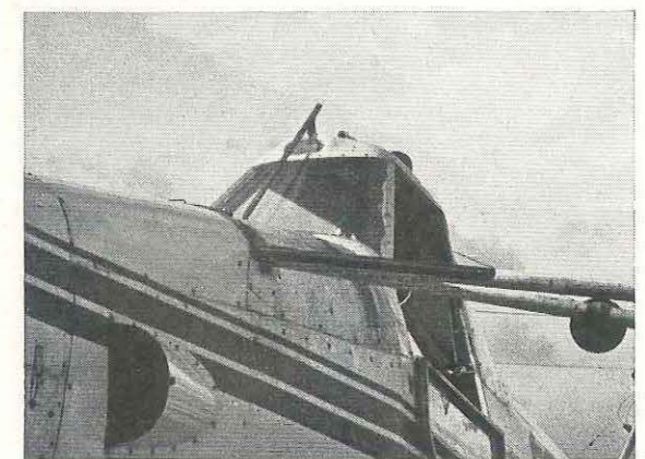
Above: Wire cutter as fitted to the windscreen of later model Pawnee aircraft.
