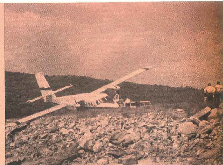
to land. (2) Aircraft loses height short of strip and in wing-down attitude strikes rock retaining wall with undercarriage and starboard wing tip. Note the dust beginning to rise. (3) Aircraft bounces up on to reclaimed area, slews to right and comes to rest in a cloud of dust. (4) Passengers evacuating aircraft after it had slithered to a stop. Strip is to the right in this picture. The starboard wing is overhanging the rock retaining wall against which the aircraft impacted.
