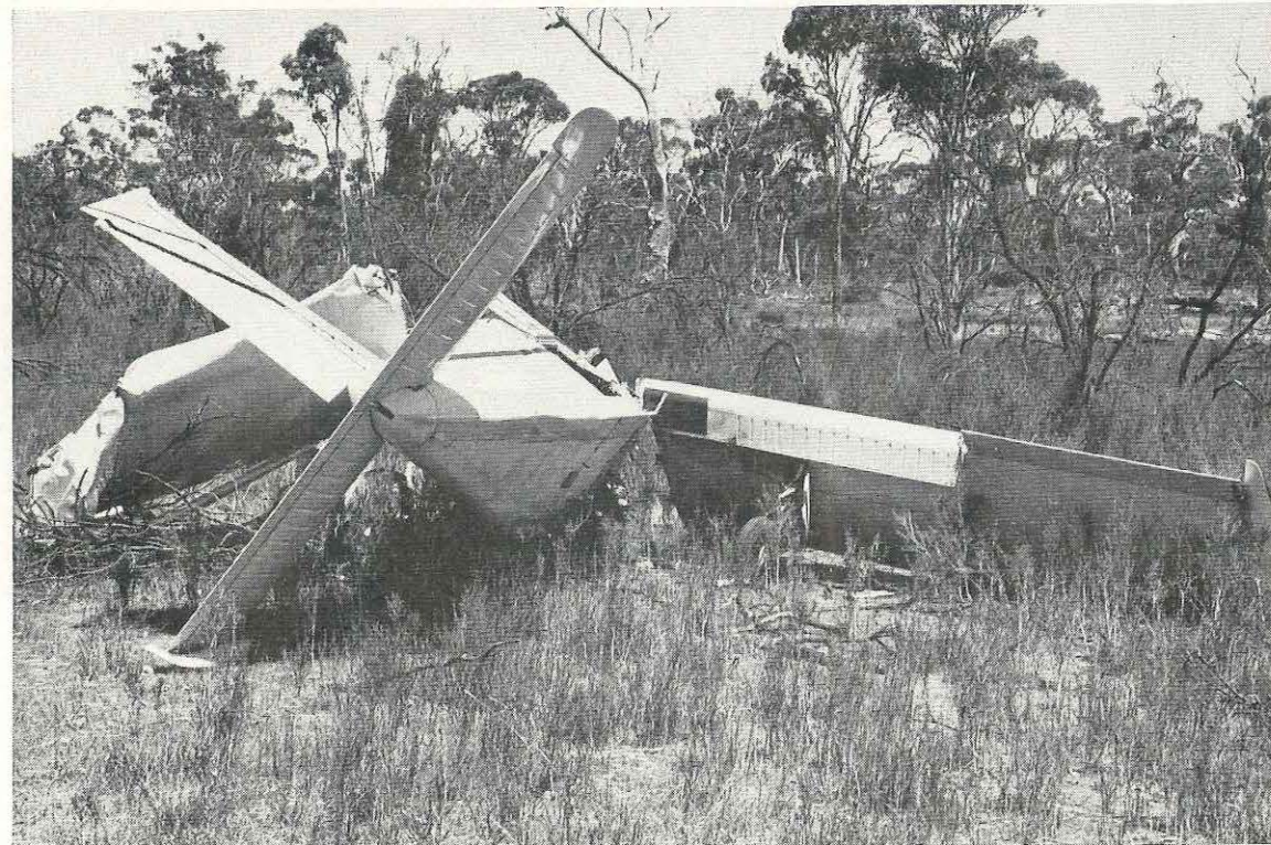
The wreckage as it came to rest. The flap position was the result of impact forces.
