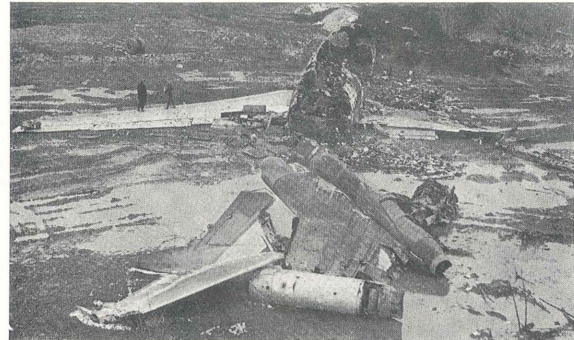
View of the wreckage showing the burnt-out fuselage and detached tail section.
