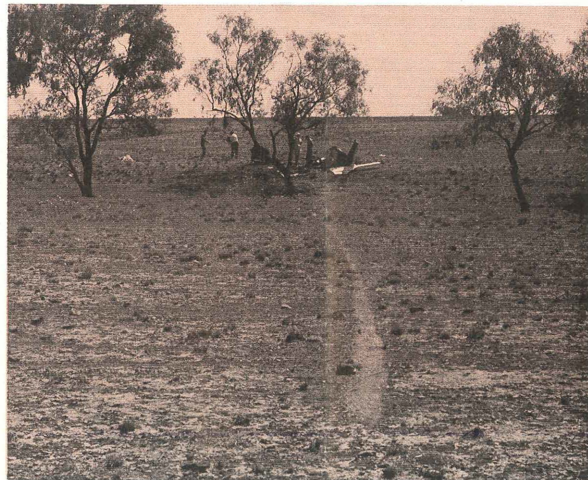
The burnt-out wreckage just beyond the line of trees in the creek bed. Note the ground mark made by the aircraft immediately before impact.
