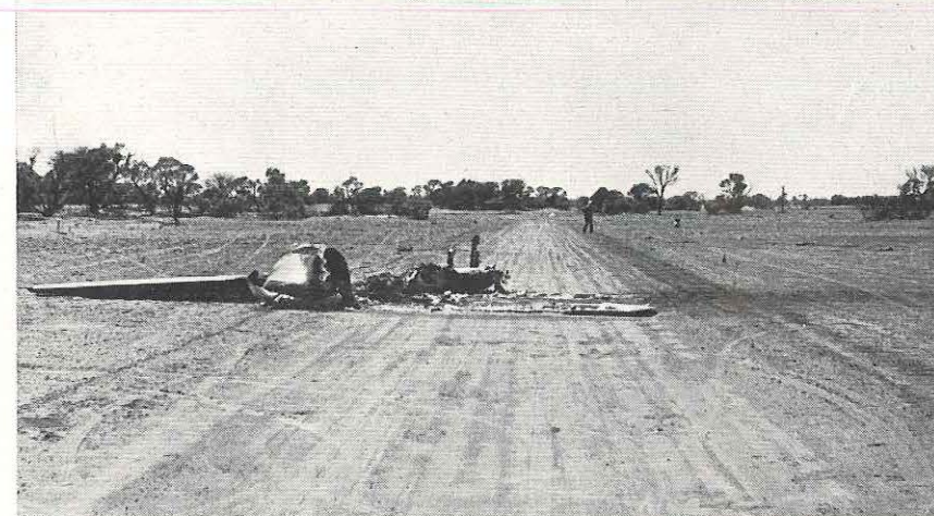
All that remained of the other Cessna 182 after the accident near Wilcannia. The pilot neglected to turn off the fuel when the nose leg collapsed.
