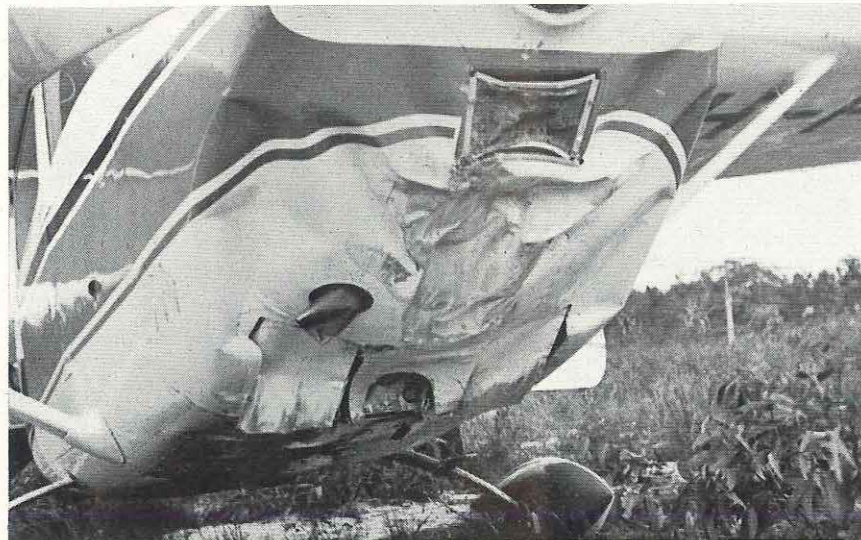
Damage to the air intake, exhaust system and the lower side of the engine compartment, where both the carburettor and fuel filter bowl are located, is clearly evident in this photograph.
