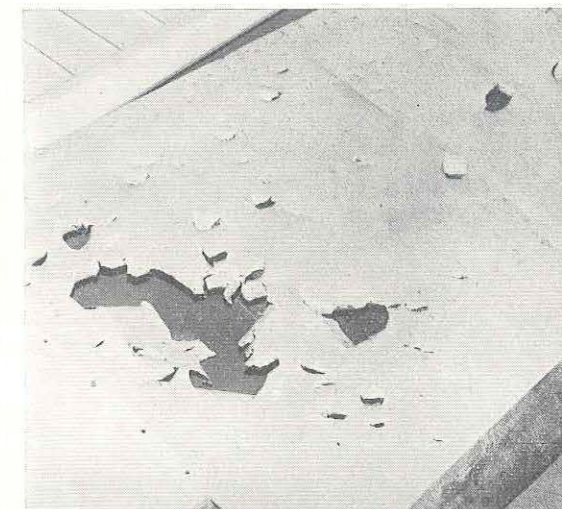
This photograph, taken after the tail plane was removed from the aircraft for repair, shows the extensive skin damage inflicted by the flailing tail wheel assembly.
