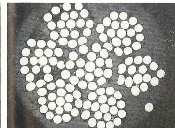
Fig. 5: Photograph of a cross section of the port cable, away from the failure area, magnified 20 times. Although wear on the surface is negligible, severe damage has already taken place within the cable.
