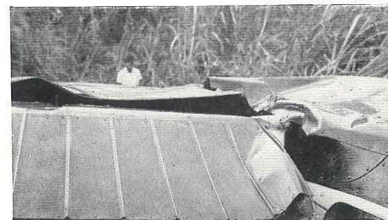
This view of the port wing root gives some idea of the very extensive damage sustained by the aircraft.
