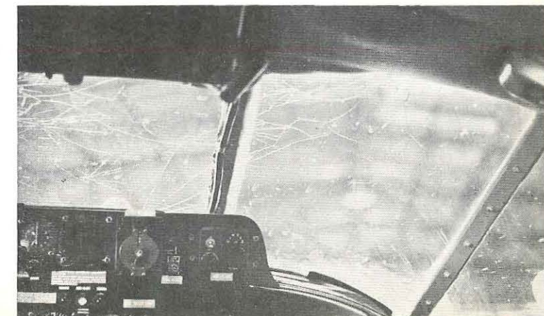
The cracked windscreen panels as seen from inside the cockpit.
