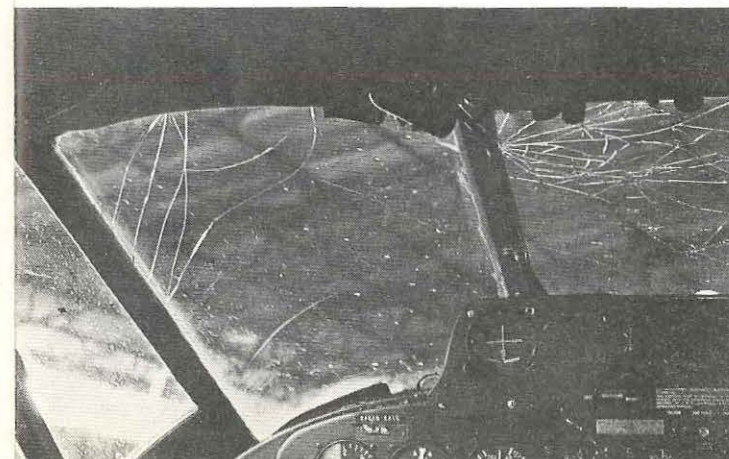
The cracked windscreen panels as seen from inside the cockpit.
