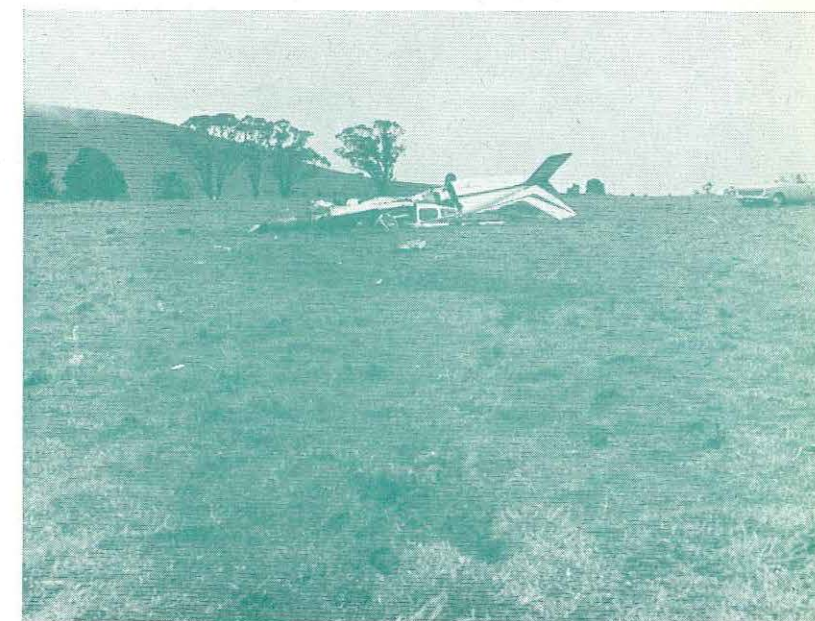
The impact marks in the foreground give some indication of the force with which the aircraft flew into the ground.
