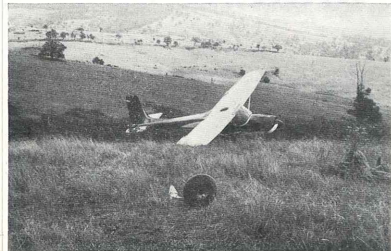
Because the rudder controls failed during take-off this Cessna 180 ran off an agricultural strip, ground-looped and was badly damaged.
