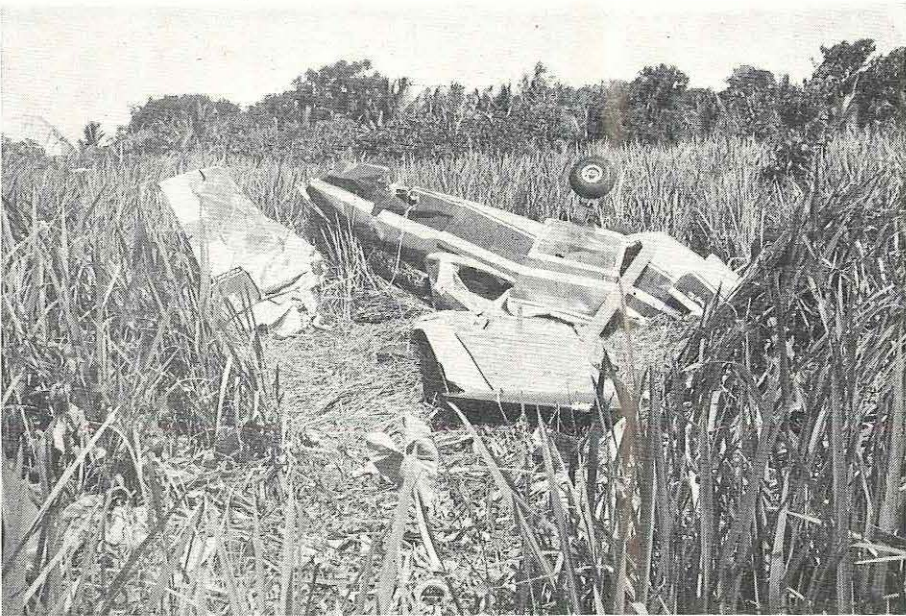
The wreckage lying where it fell in kunai grass. The tail assembly is separated from the fuselage and held only by the control cables.
