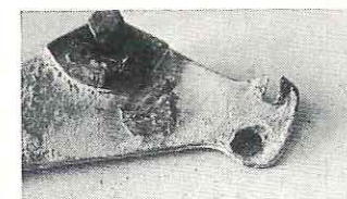
Below left: The rubber bell-crank on the port side, though still intact, was also found to be badly worn.
