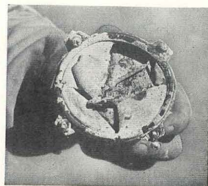
The engine tachometer as recovered from the wreckage. The needle is jammed in the 2,500 r.p.m. position.
