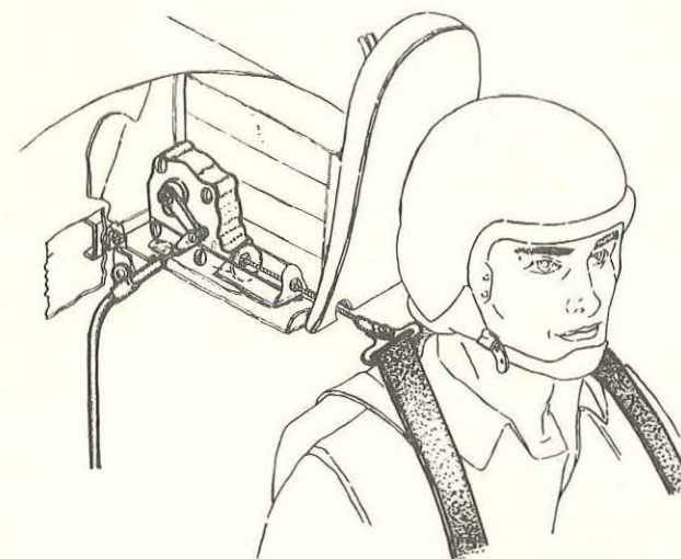
FIG. 1. TYPICAL PILOTS INERTIA REEL-SHOULDER HARNESS INSTALLATION.
