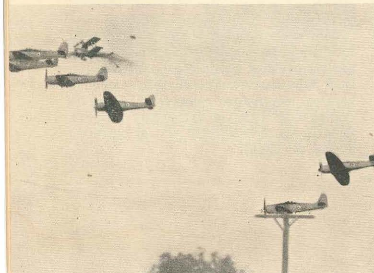
In the view below the formation leader has just hit the DH.82 with propeller, canopy and fin whilst Nos. 4 and 6 continue breaking away. In the view above the DH.82 is seen disintegrating further whilst the damage to the leader's fin and rudder is visible.
