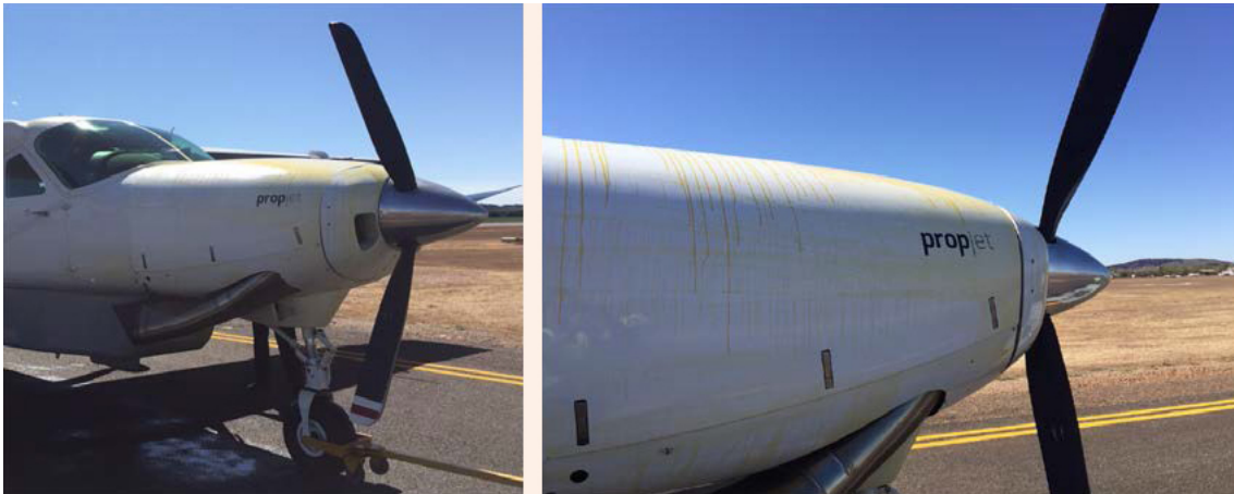
Figure 13: Photographs of VH-LNH after the aircraft had landed, with oil visible on the engine cowl and forward fuselage.
