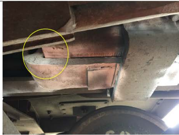
Figure 3 Yoke with no relief fillet
