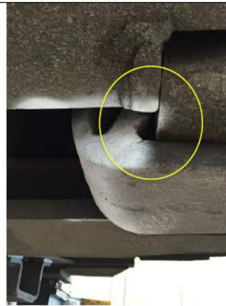
Figure 4 Yoke with relief fillet
