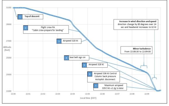
Figure 1: Diagram showing actions, conditions, and events during the aircraft's descent
