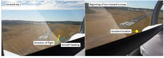
The figure shows images of the aircraft during the approach prior to the accident. The aircraft is shown in a forward slip (left) and at the beginning of the turn toward the runway 05 threshold (right). Source: Passenger, annotated by ATSB
