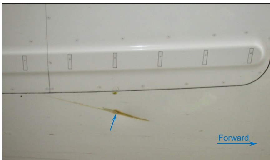
Figure 4: Contact mark below rear cargo door
