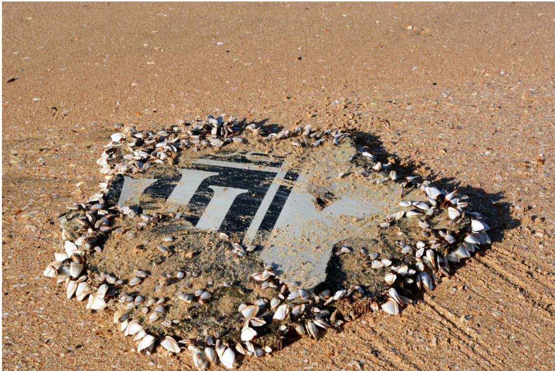
Figure 3: Photograph taken 23 Dec 2015 showing Part No. 3 significantly colonised by barnacles
