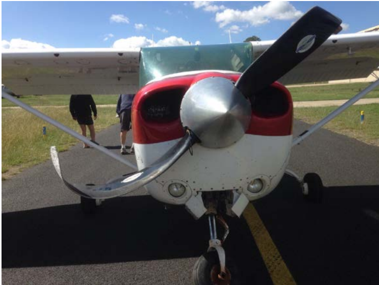
Figure 1: VH-JXX showing damage to the propeller and nose landing gear
