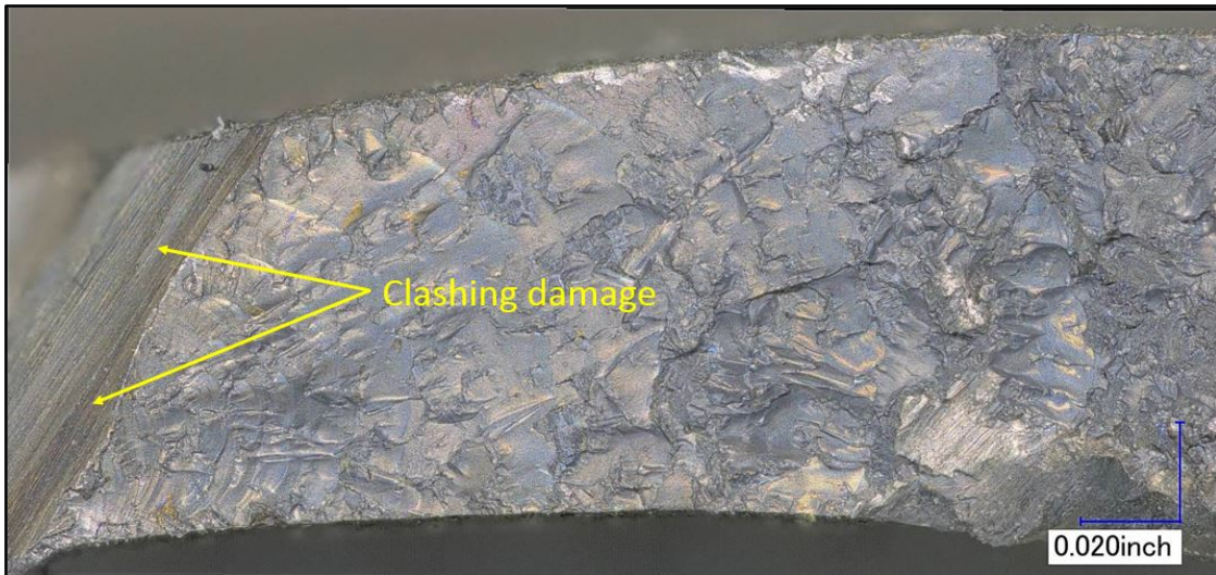
Figure 7: Blade 120 fatigue region, with leading edge clashing damage indicated on the left
