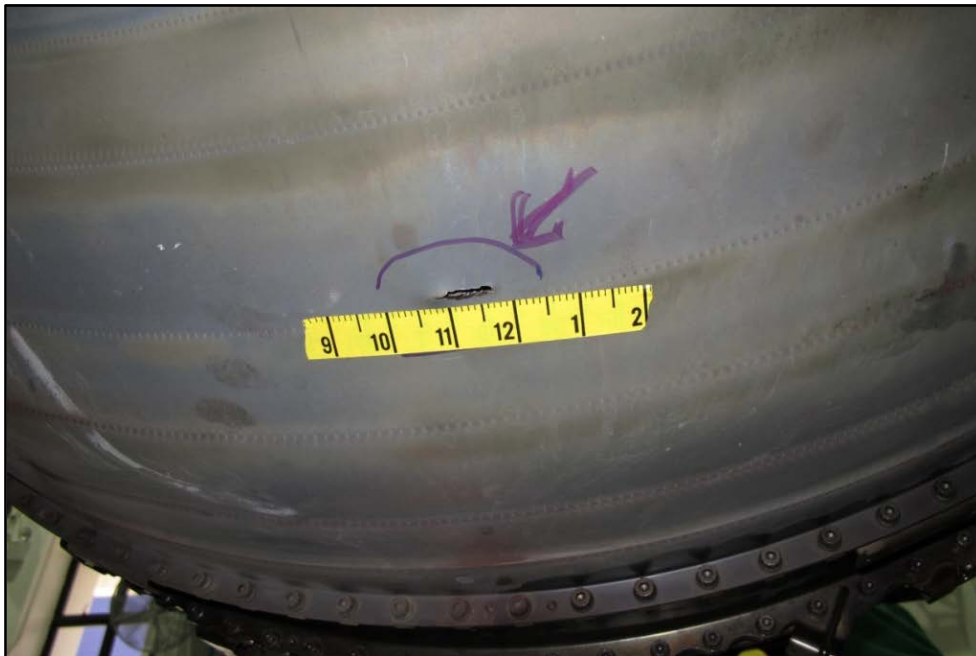
Figure 11: Low-pressure turbine front case tear at the 6 o'clock position. Note that the scale is in inches and the view is looking aft
