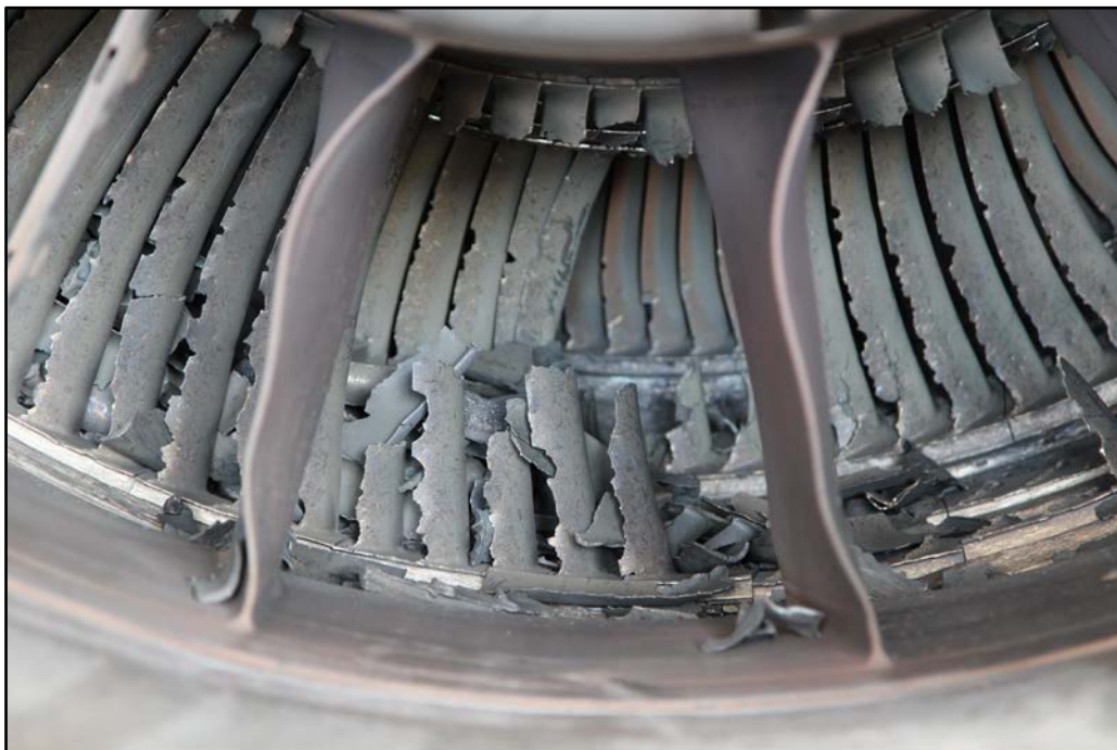
Figure 2: Right engine low-pressure turbine damage, looking forward from the exhaust duct
