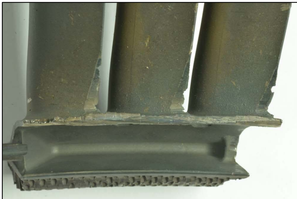
Figure 12: Stage four low-pressure turbine vane cluster showing clashing damage to the inside diameter of the shroud and aerofoils
