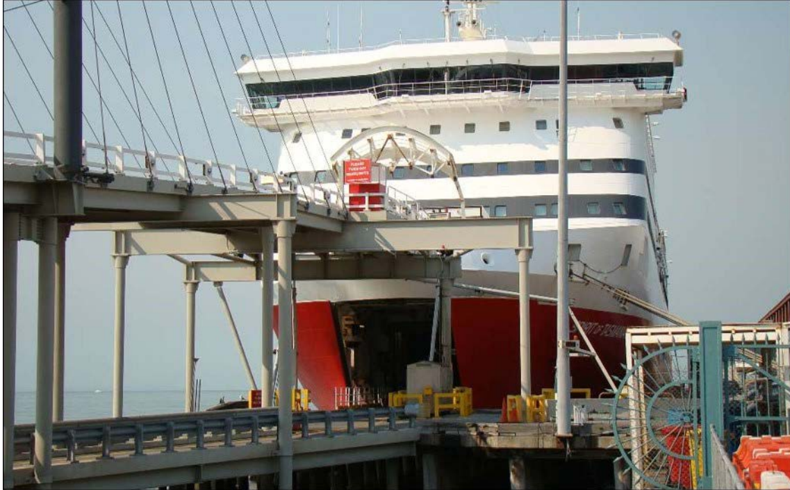
Figure 1: Spirit of Tasmania II 's upper and lower bow ramps deployed at Station Pier
